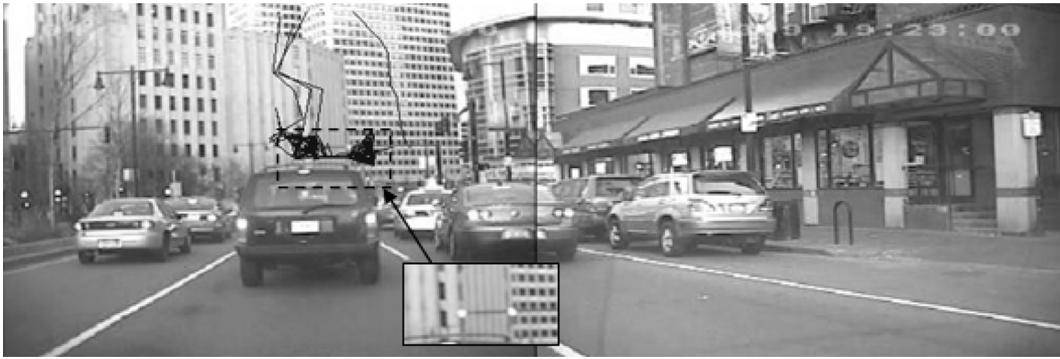
Fig. 13. A trace of the calculated telescope aiming points while the driver was stopped for a red light. It clearly shows that the driver monitored the lights through the bioptic telescope. The inset, on the lower right of the left camera image, is added here to reveal the area obscured by the dense aiming points.
