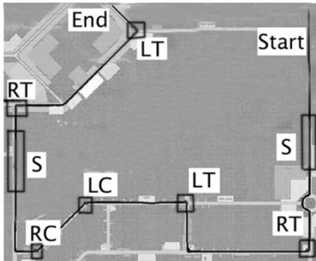
**Figure 2:** A typical route for a scripted city drive showing the locations of the road segments selected for the analysis of vehicle handling skills and head movement behaviors. Segments were selected such that they were free of any traffic situations or pedestrian appearances that might affect the skills (lane positioning, steering) being assessed. S = Straight segment; RT/LT = Right/left turn; RC/LC = Right/left curve.
