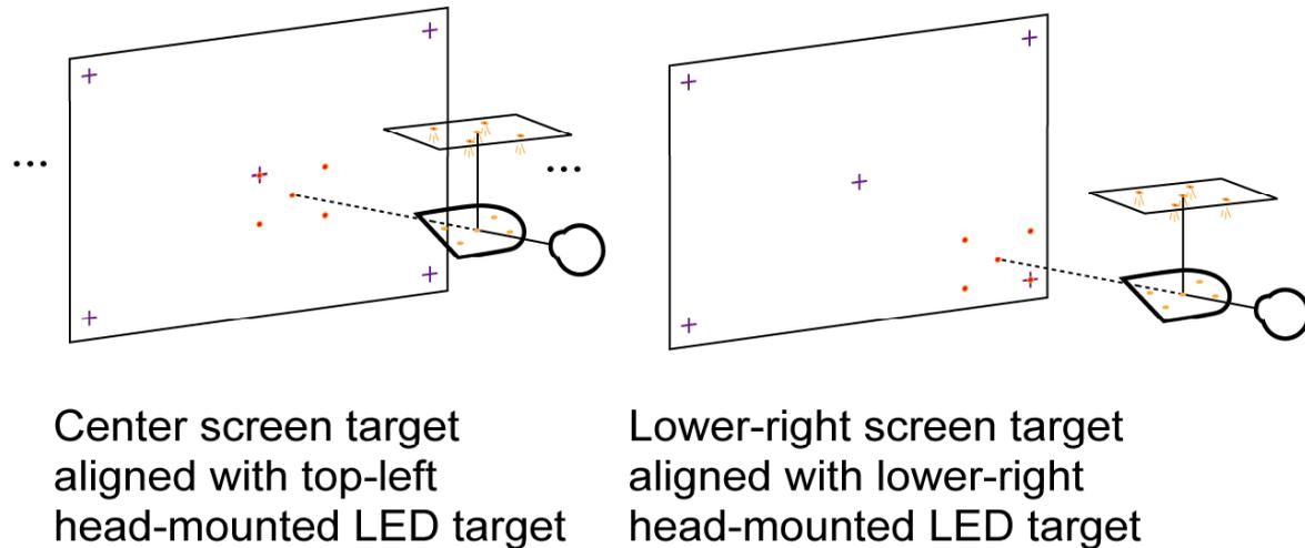
**Figure 4:** Geometric calibration procedure. Subject aligns combinations of head-mounted and screen targets.
