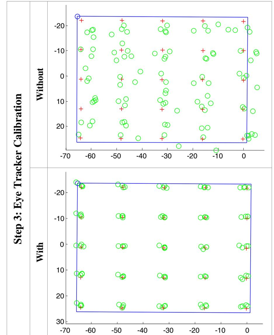
**Figure 8:** Model-predicted screen intersections of gaze line with and without eye tracking. Data for 100 gazes each from a different viewing location. Motion tracker transmitter was moved closer to measurement space (fig. 6)
