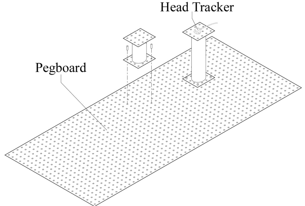
Figure 3: 3D Pegboard system for placing tracker at known locations
