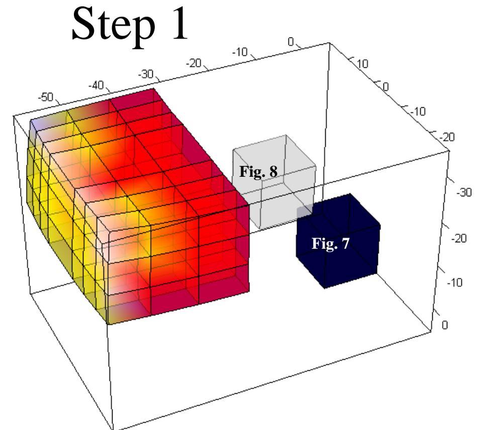
**Figure 6:** Distortion measured in calibration step 1. Plot shows reported locations of head tracker when placed at 128 locations on 3D pegboard. Units are inches in coordinate system of head tracker transmitter (black cube). Yellow areas have error of up to six inches.
