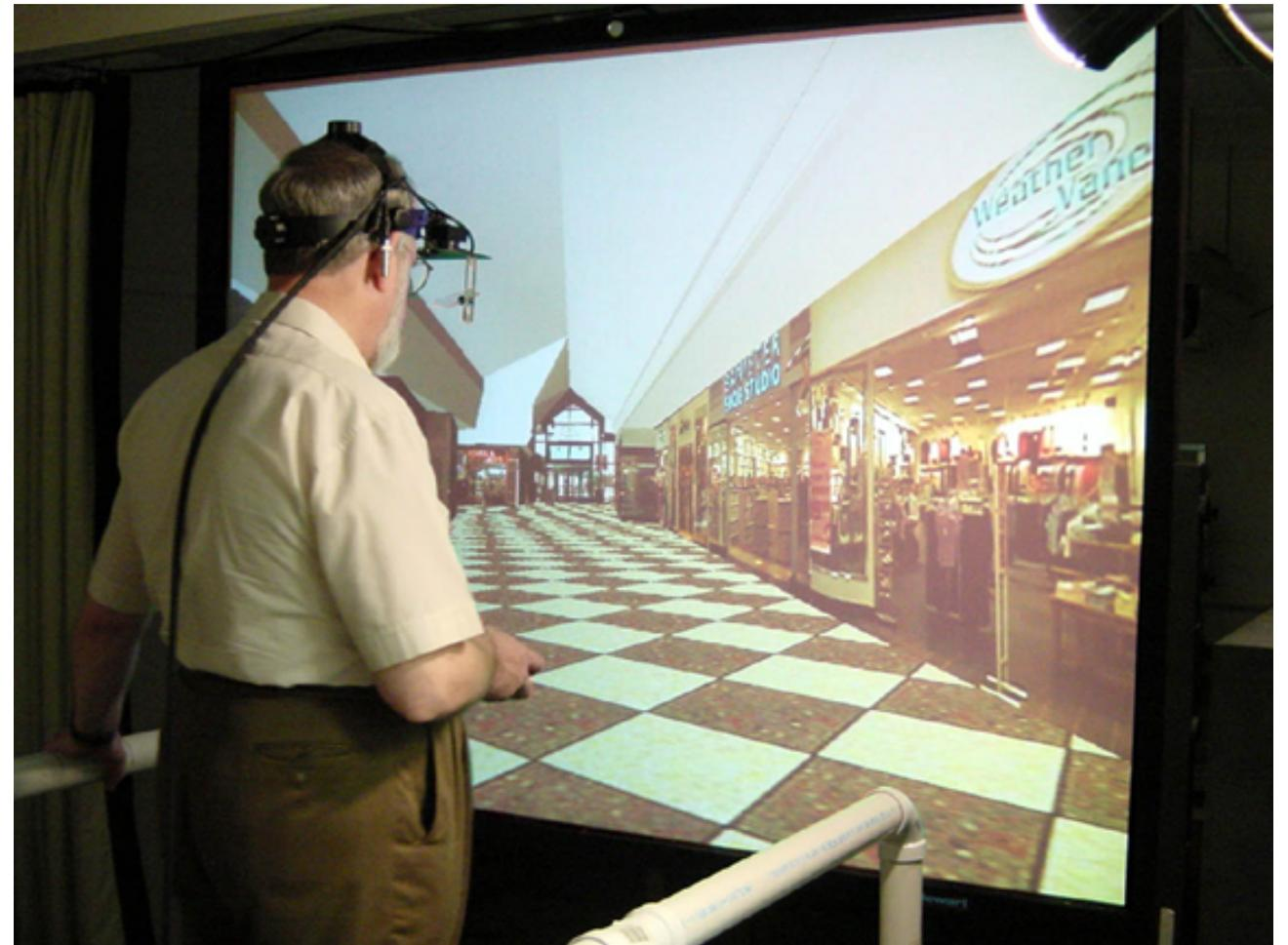
**Figure 1:** Subject viewing virtual environment while standing on a treadmill. Screen spans  $85^\circ$  at a distance of 36"
