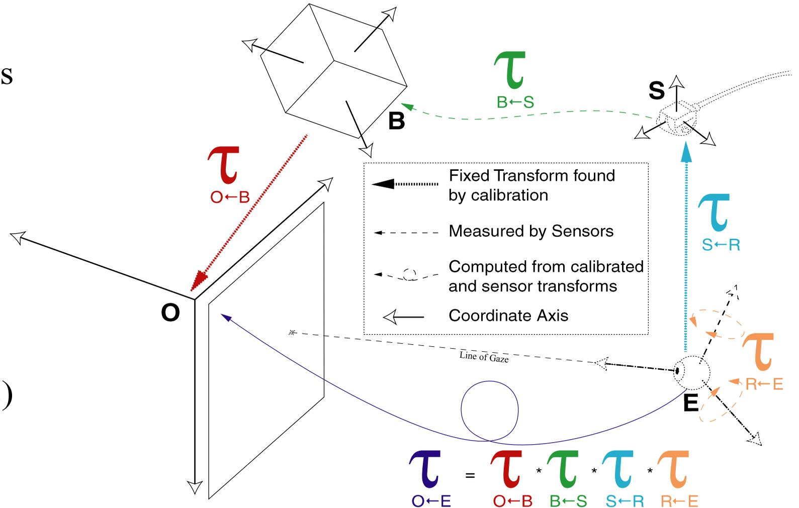
**Figure 2:** Geometric Model Used to Find Gaze Frame
