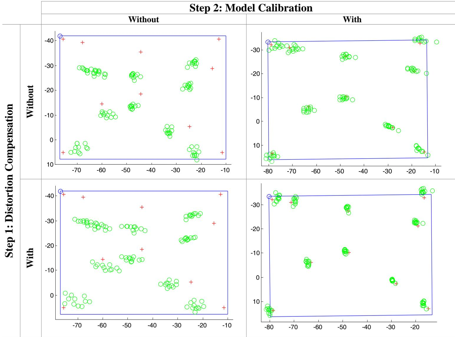
**Figure 7:** Model-predicted screen intersections of gaze line omitting calibration steps one and/or two for subject looking through center ad-mounted LED target (no eye movement). Axes are labeled in coordinate system of head tracker transmitter, units are inches. Red crosses are actual gaze point. Green circles are predicted gazes from eleven viewing locations.
