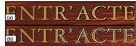
(a) Example of new filter (b) Previous (?=?) filter The edge ringing was especially noticeable on text.
