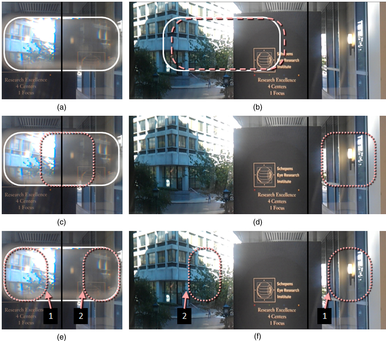
Fig. 14 Photographed view through a 57 \Delta EPS base-left Fresnel prism. The vertical line in each figure is at 0 deg (PG) incidence angle. (a) The view through an EPS prism is outlined. The entire view is less distorted than with OPS, but reflections affect both seeing and blind hemifields. (b) The same view without the prism. The solid outline indicates the area that would be viewed in a prism with CDA, whereas the dashed pink outline indicates the area seen directly in the EPS prism. Magnification results in a narrower field seen through the prism view than with CDA or the OPS shown in Fig. 13, but without the pronounced distortion and TIR light loss left of center that affects OPS. However, the entire view is compromised by bright reflections. (c) Reflections on the bases (R) superimpose a strong mirror image of the bright area (lamp and glare on the window) to the right in (d) and cause monocular visual confusion. (e) Dimmer SRs from the area marked 2 (shaded part of building) outlined in (f) superimposes an almost see-through view in the primary seeing hemifield, causing monocular visual confusion (seeing the part of the brochure and bright building at the same direction) and reduced contrast for the intended brochure view. But, the surface reflection from the area marked 1 (area around the lamp) will fall on the blind hemifield. When the patient scans leftward, the area marked 1 (including the lamp) causes monocular visual confusion with the bright building from the intended image, and the area marked 2 causes diplopia (shaded part of the building seen twice; once dim in SR and once bright in the intended image on the blind side).
