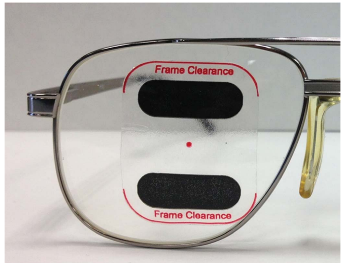
FIGURE 4. The fitting template for peripheral prisms. A seemingly simple device that highly simplifies the fitting procedure by setting the prism position, simultaneously ensuring that the permanent prisms can be safely embedded into the carrier lens and marking a 3-mm safety margin around the prism. Note the crucial tangential point at the nasal edge of the lower segment. This helpful template was developed by Charlie Saccarelli, President of Chadwick Optical.
