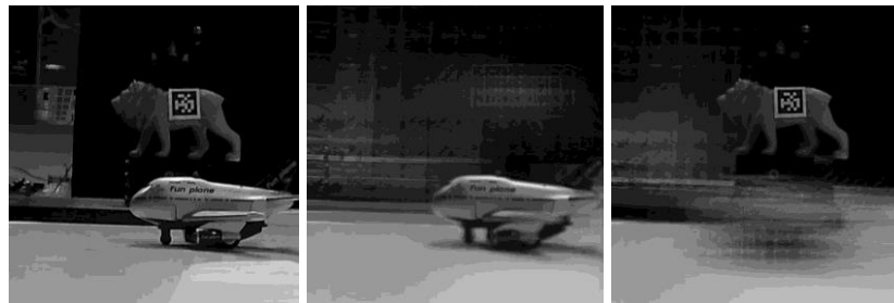
Fig. 2. Cropped reconstructed depth-plane images in the detected peaks of the average gradient magnitude of the CII reconstructed image planes. Left: original scene. Middle: reconstructed image at a depth of 280 mm from the camera. Right: reconstructed image at a depth of 600 mm from the camera. The airplane and lion toys were placed 280 and 600 mm away from the camera array, respectively.
