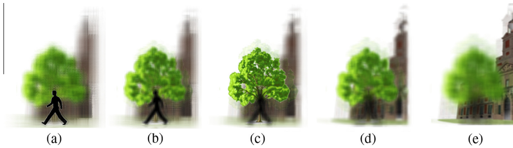
Fig. 11. Confocal images ( 308 \times 385 ) in different depth planes generated from a simulated elemental image frame obtained computationally (Fig. 10) from the simulated 3 plane scene of Fig. 1. (a) The confocal images at the depth plane of the pedestrian (1 m), (b) between the pedestrian and the tree (2.5 m), (c) of the tree (4 m), (d) between the tree and the building (6.5 m), and (e) of the building (9 m). Animation 1 in the online supplement shows the confocal image sequence being scanned between near and far in depth.
