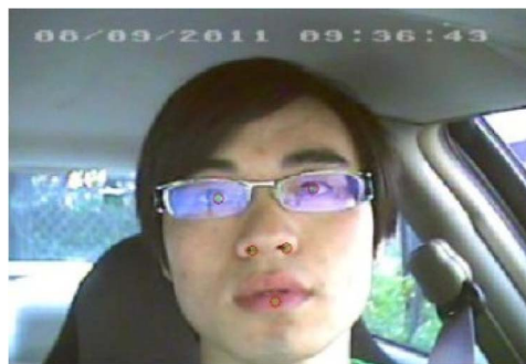
Fig. 4. Successful facial feature detection [28] used to enhance the accuracy of gaze estimation is shown as circles marking the lower lip, the nostrils, and the irises.
