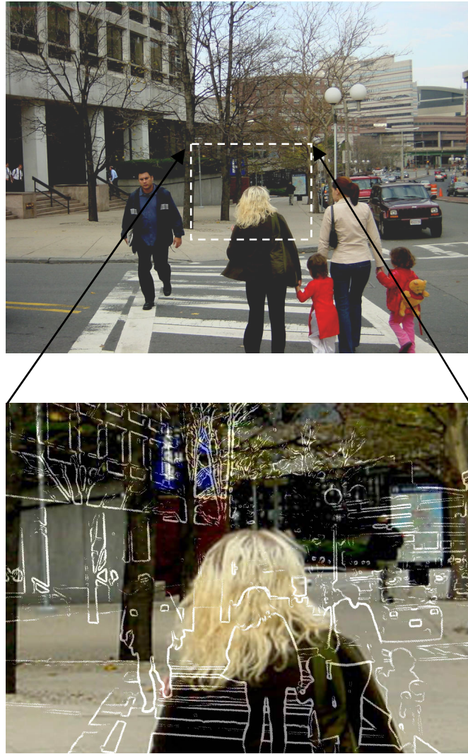
Figure 1. Illustration of the augmented view provided by the HMD system. The upper image shows a full view of a street scene captured by the camera of the system. The white rectangle inset represents the size of the field of the display. The lower image shows a minified edge of the scene (enlarged here for clarity) superimposed on the natural see-through view.
