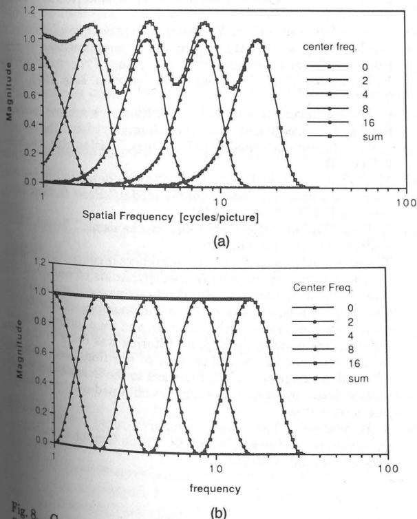
Fig. 8. Comparison of Gaussian (Gabor filters) with the cosine log filters used here. (a) Filter bank of 1-octave-wide Gaussian filters and the sum of all filters. (b) Filter bank of 1-octave-wide cosine log filters. Here the summation of all the filters adds to the unity. Note also the symmetry of the cosine log filters on a logarithmic scale.
