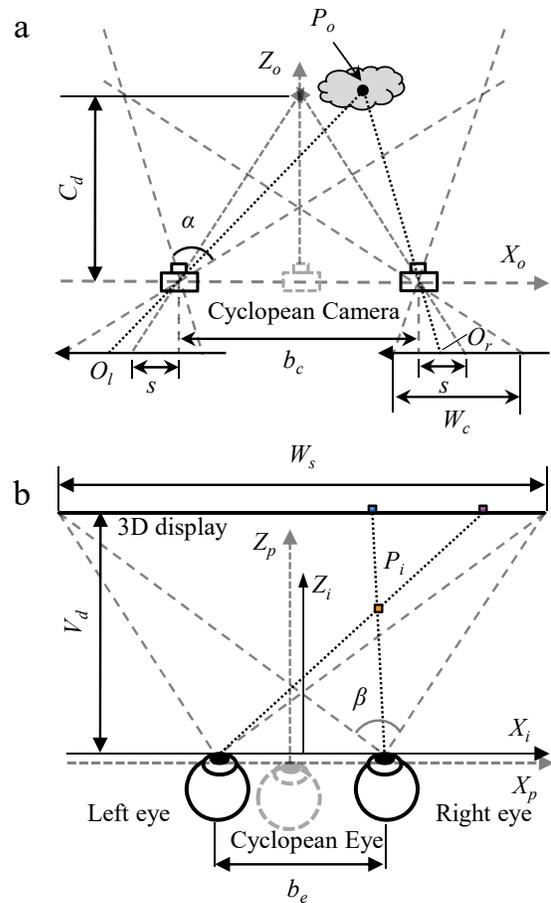
**Figure 3.** VR content acquisition, display and perception. (a) Natural world scene acquisition with parallel camera configuration; (b) virtual world presenting and perception. See Table 2 for symbols' meaning.
