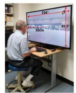
**Figure 4:** Experimental setup. A large display  $(104^{\circ}H \times 81.5^{\circ}V)$  is placed on a height-adjustable table to align the subject's eye level with the screen center. The rendering camera's field of view and display field of view were matched. Subjects were instructed to press a key if an approaching pedestrian appeared to bump into them.
