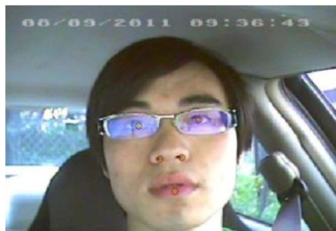
Fig. 4. Successful facial feature detection [28] used to enhance the accuracy of gaze estimation is shown as circles marking the lower lip, the nostrils, and the irises.
