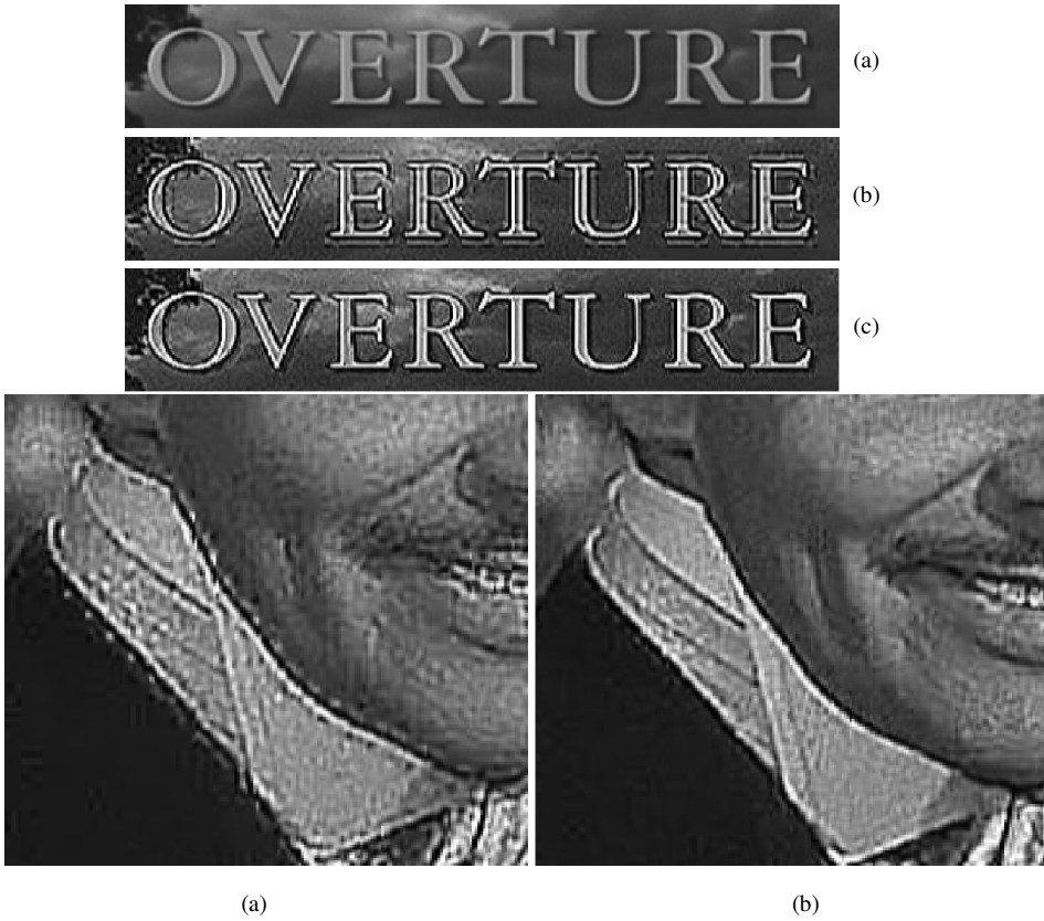
Fig. 5. Illustration of ringing artifacts and their reduction in the MPEG enhancement. 21 (a) Unenhanced section of a movie frame with text. (b) Text is particularly prone to ringing artifacts caused by enhancement that is limited to a band of frequencies in the DCT block. (c) Our recent filtering techniques have substantially reduced these ringing artifacts without reducing the contrast enhancement effect. (d) Curved edges appear ‘jagged’ when ringing artifacts are caused by the DCT filtering. (e) The more recent filtering applied has reduced these artifacts.
