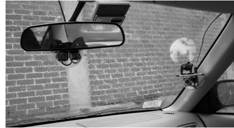
Figure 2 The digital in-car surveillance system is comprised of one scene camera aimed at the road ahead and two cameras aimed at the driver.
