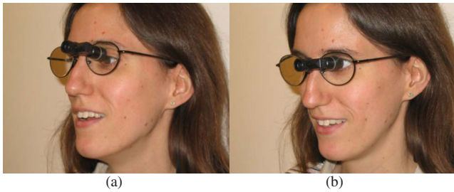
Fig. 1 A monocular Keplerian bioptic telescope. (a) Most of the time the wearer views through the carrier lens without any effect of the telescope. (b) With a slight downward tilt of the head, the telescope is brought into the line of sight, enabling a magnified view of the object of interest. The telescope shown is the 3× mini focusable Keplerian bioptic manufactured by Ocutech, Incorporated (Chapel Hill, North Carolina).
