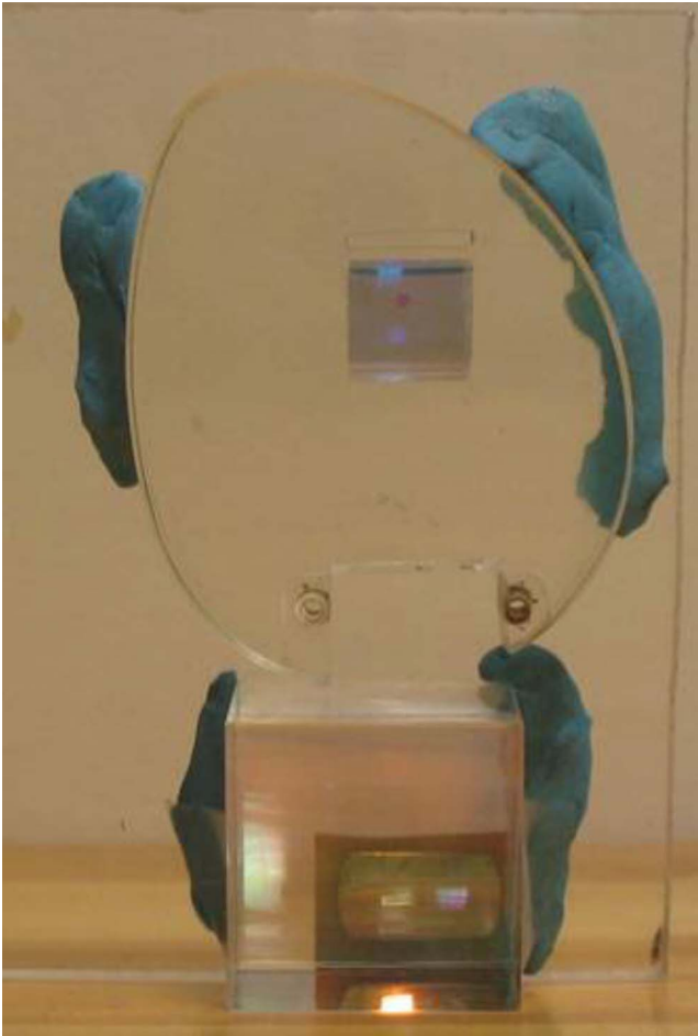
Fig. 12 A prototype implementing an astronomical Keplerian telescope using polarizing beamsplitters and spherical mirrors. The objective assembly (top) is composed from the magnifying element of a MicroOptical display system, which includes a polarizing beamsplitter, a quarter-wave plate, and a spherical mirror (top). The ocular assembly (below) is constructed from a polarizing cube beamsplitter, a quarter-wave plate, and a conventional plano-convex lens that was silvered on the convex surface. A dark occluder is visible behind the image of the ocular spherical mirror.
