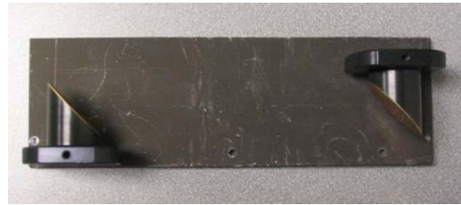
Fig. 8 An astronomical Keplerian prototype telescope constructed from two 90-deg off-axis parabolic mirrors.
