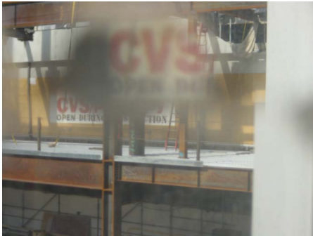
Fig. 6 An image photographed through the first prototype shown in Fig. 5. The magnified image of the CVS sign is shown above and to the right of the nonmagnified view of the sign obtained through the carrier lens, illustrating spatial multiplexing by shifting. The shift was obtained by tilting the whole lens assembly relative to the camera, which resulted in a blurred magnified image.
