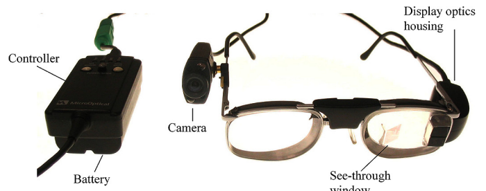
FIGURE 3 — The current generation of the augmented-vision HMD visual field expander for patients with tunnel vision. The wide-angle image captured by the video camera is processed by the controller to provide edge-contour images of the scene. The edge images are displayed on the see-through display providing an expanded view. Once an object is detected via the minified cartoon, it can be examined with full resolution and color through the transparent display.
