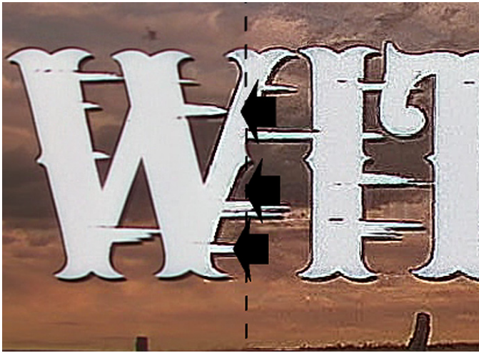
FIGURE 6 — This frame illustrates partial screen enhancement (to the right of the dashed line) and a situation (letters moving leftward) where partially enhanced macroblocks appear on the unenhanced section of the frame. Predicted blocks based on an enhanced reference from the right side of the line appear moderately enhanced on the left side of the line. The area where the effect is most obvious has been indicated with arrowheads. The dividing line has been added for clarity of the illustration; it does not appear on the screen.
