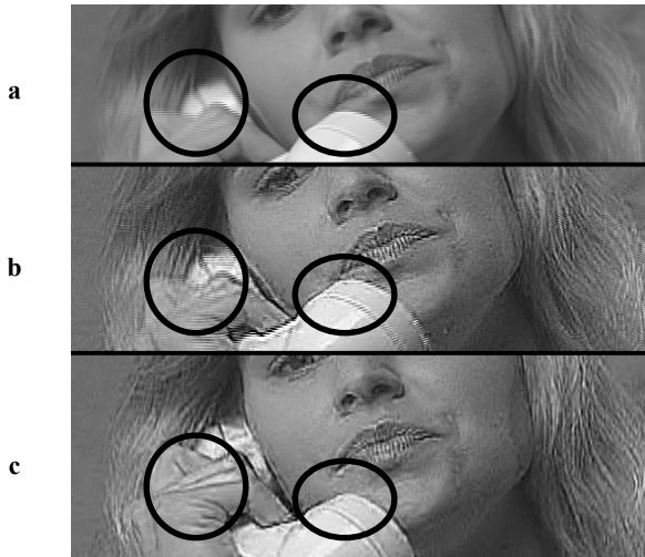
Fig. 5. Enhancement and reduction of interlacing artifacts. Shown are three segments of frames from a motion event. Areas where the effect is particularly prominent have been circled for emphasis and comparison. (a) Interlacing artifacts caused by the combination of two fields from two different instants in time. (b) Enhancement ( \lambda=4.0 , \alpha=1.5 ) without deinterlacing accentuates these artifacts. (c) Using VLC 'linear' deinterlacing filter reduces these interlacing or "motion" artifacts.
