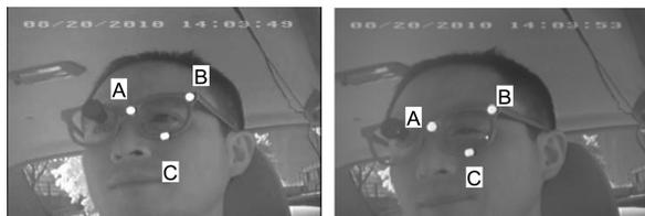
Fig. 8. When making a downward head tilt to look through the telescope, the angles of the reflective marker triangle change. The angles are used to estimate the telescope aiming point.
