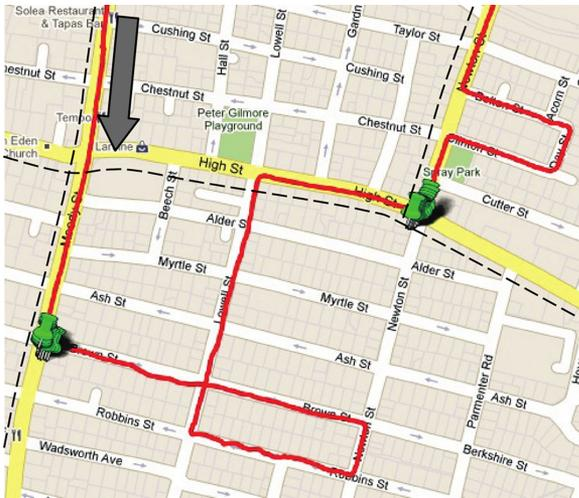
Fig. 5. Detection of left turns on major roads (shown in yellow and highlighted with dashed lines) by filtering left turn detection results with road class data at intersections. Note that the two left turns at minor intersections are not flagged, nor are the right turns.
