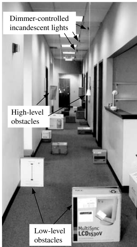
Figure 3. One of the two corridors on the indoor obstacle course. The illumination level was adjusted by dimmer controlled incandescent lights. The bright fluorescent lights seen in the picture were only used to take this picture.
