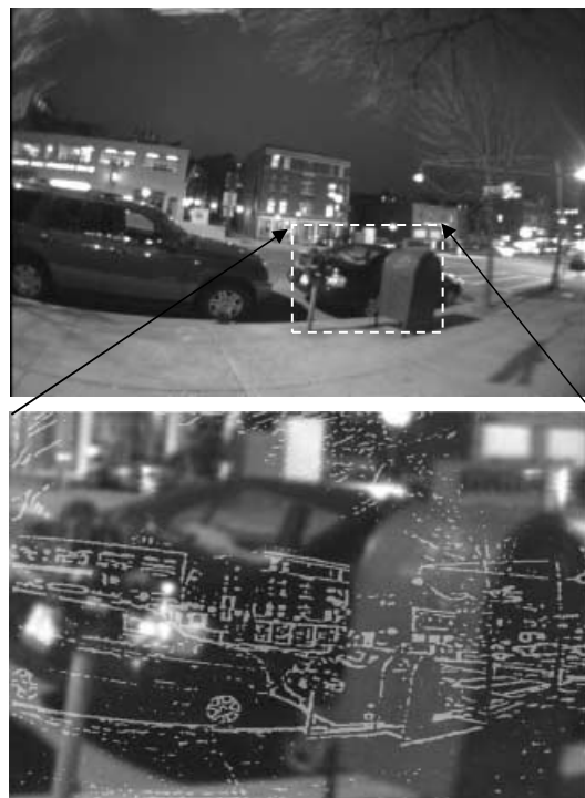
Figure 1. Illustration of the Augmented-View concept. The upper image shows a full view of a street scene taken at night with the camera used in the LV-3 device; the white rectangle inset represents the size of the field of the display. In the partial implementation of the concept (Minified Augmented-View) used in the prototype LV-3 device, a minified gray-scale image of this scene was presented on the device display. The lower image shows the Minified-Contours Augmented-View concept that will be implemented in future versions of the device, where a minified edge-contour image of the scene (shown here without minification) will be superimposed on the natural see-through view (shown here as the car and mail box, etc. behind the edge-contour image). For the purpose of illustration the edge-contour image is shown over the image obtained with the night vision camera; however a person with night blindness at low light levels would see less detail with their natural vision.
