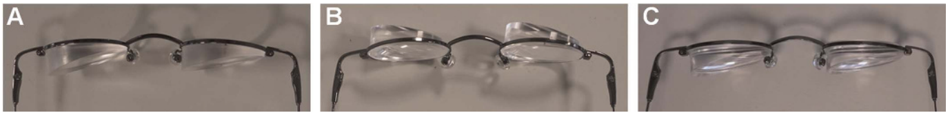
FIGURE 3. Pictures of full-field prism configurations ( 12\Delta yoked prisms). (A) Meniscus full-field prisms mounted with the bevel positioned at the front surface. (B) Flat full-field prisms with bevel positioned at the back surface to mount to the frame (outward prism serration). (C) Flat prisms mounted with bevel positioned at the front surface (eyeward prism serration). Note that the prisms were mounted in a special frame with very narrow eyewire to reduce the thickness of the prism base.
