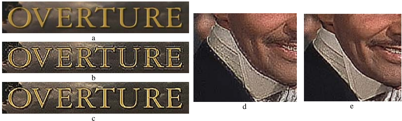
Fig. 5. Illustration of ringing artifacts and their reduction in the MPEG enhancement [21]. (a) Unenhanced section of a movie frame with text. (b) Text is particularly prone to ringing artifacts caused by enhancement that is limited to a band of frequencies in the DCT block. (c) Our recent filtering techniques have substantially reduced these ringing artifacts without reducing the contrast enhancement effect. (d) Curved edges appear ‘jagged’ when ringing artifacts are caused by the DCT filtering. (e) The more recent filtering applied has reduced these artifacts.
