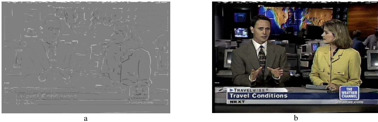
Fig. 4. Wideband enhancement. (a) Bipolar features (edges and bars) detected from the original image are scaled according to the strength of the feature. (b) The bipolar features added to the original image. Note the white line on the woman's left arm. The features brightness can be adjusted to increase or decrease the level of enhancement.
