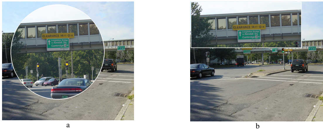
Fig. 6. Simulated view of a road sign viewed through a 3.0 \times telescope. a) The view through a conventional binocular bioptic. The magnified image on the retina blocks the view of much of the intersection, creating a ring scotoma (blind area). b) Spatial multiplexing by shifting. The rectangular field of view through the in-the-lens telescope described here. The magnified image is shifted up, blocking in part the view of the pedestrian bridge overhead but leaving the traffic in the intersection in full view. Note the non-magnified view of the road sign seen under the magnified view. The white line surrounding the magnified images is added only for clarity of these illustrations.
