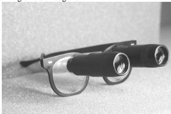
Figure 1: A binocular Keplerian bioptic telescope. The device is mounted at the top of the spectacle lens and is slightly tilted upwards.
