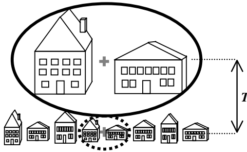
Figure 6. Simulvision concept. The magnified (solid line oval) is angularly displaced to permit the direct view of the unmagnified object (dotted line oval).
