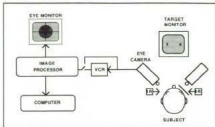
FIGURE 1: A schematic of the video-based eye movement recording system used in the present study. Eye movements were recorded using only one camera at a time; the fellow eye was patched.
