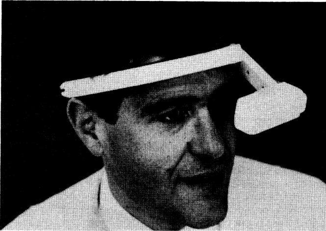
Fig. 1. The display is positioned in front of one eye using an adjustable headband. The other eye continues to view the environment.
