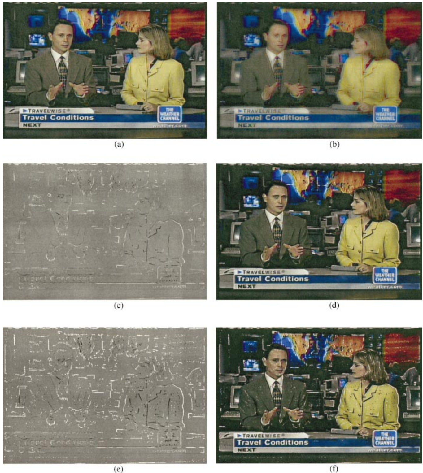
Fig. 2. (a) Original image. This TV image was particularly sharp and had high signal-to-noise ratio. (b) Degraded image processed with the Adaptive Enhancement algorithm 1 with K = 0.37 . (c) The bipolar edge and bar features of various strengths detected from the original are shown at scale factor 255 (level 9 in Table 1); they were then added to the original image to create the enhanced image in (d). (e) Shown at scale factor 3199 (level 15 in Table 1) are the bipolar edges of various strengths detected from the original that were then added to the original image to create the enhanced image in (f). The selected median enhancement level 7 from 35 patients in procedure 1 was not clearly visible in print even though it was clearly visible on the TV monitor. The high enhancement level shown in (e) and (f) is equivalent to enhancement done with binary substitution.
