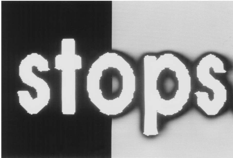
Fig. 1. Examples of unenhanced (left) and enhanced (right) text. Subjects never saw the two conditions on the same screen. Note the increased size of the enhanced text, which is due to the dark annular region around each character.
