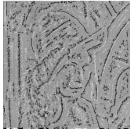
Fig. 4. Features map derived from the images in Fig. 2 using the same congruence rule as in Fig. 3, but dropping the lowest scale image (order three). When compared to the features map in Fig. 3, this demonstrates a higher rate of feature detection, but also a significant increase of false alarms or noise pixels.
