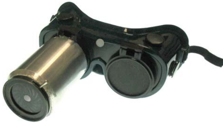
Fig. 3. Goggles used by control subjects in restricted-vision trials. The adjustable iris on the extension tube was used to match the field size of each patient. Control subjects paired with patients with acuity 20/40, or worse, had their vision blurred by layers of sandwich like plastic added until their vision was within one line of their patient's on a Snellen chart viewed at 1 m (to approximate the distance they would be viewing the VR screen). An opaque disc in the left eyepiece obscured vision by that eye. The iris opening in the photograph is set for the control subject with a 5° restricted field of view. The extension tube was necessary to avoid a pinhole magnification (diffraction) effect at the smallest settings.
