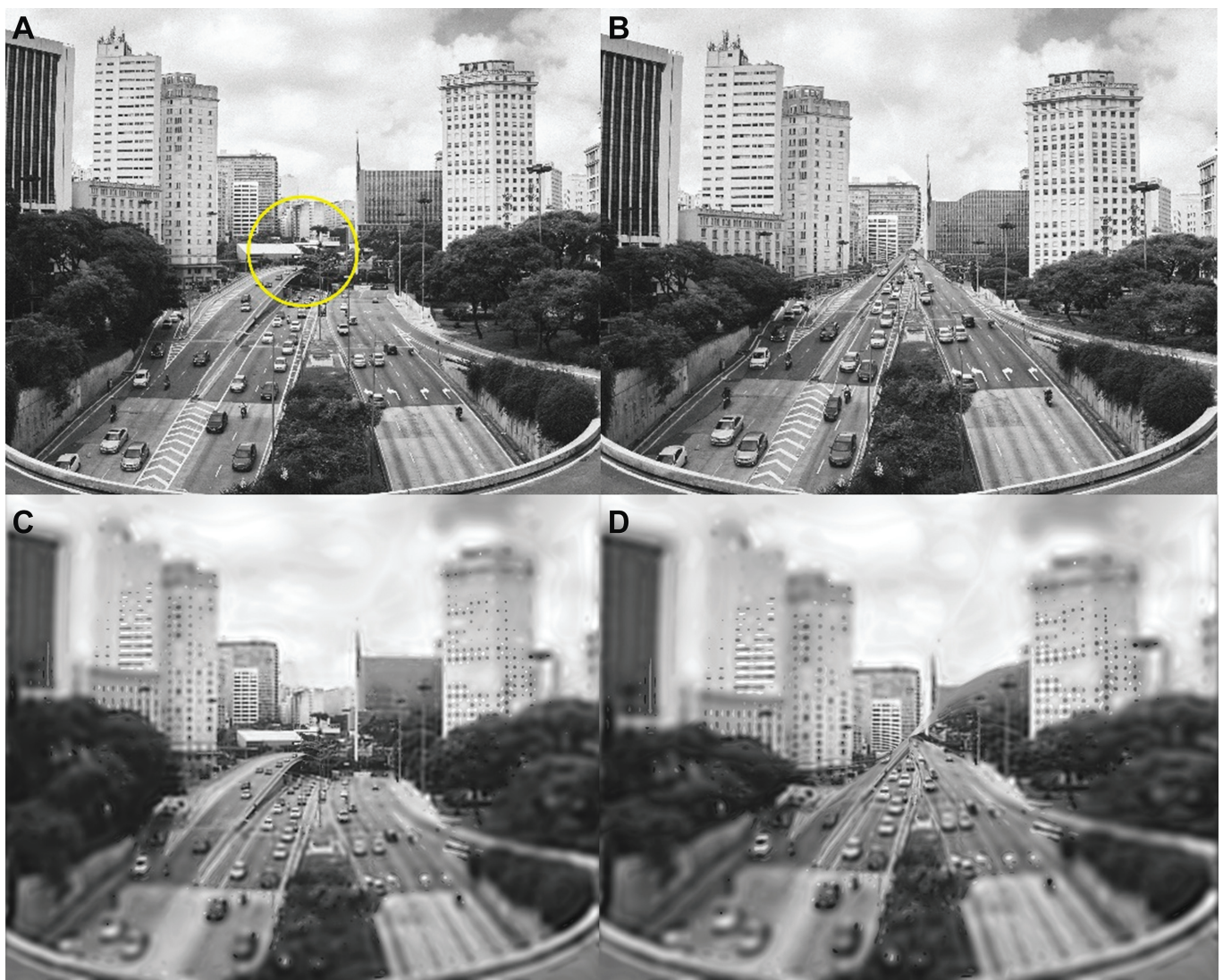
FIGURE 6. Central scotoma carving. (A) A scene spanning 32° with the location of a 6° central disciform scotoma marked (yellow circle). (B) Alternating scotoma carving. Applying vertical seam alternating with horizontal seam to the original scene in (A). Distortions are apparent in comparing the images in (A) and (B), but the image in (B) is completely acceptable if examined without comparison. (C) The original image in (A) was processed with the Peli model to simulate the decline in resolution and contrast sensitivity with retinal eccentricity. 32,43 (D) The image in (C) after alternating scotoma carving representing the view of a patient with a disciform scotoma. The most notable effect is the “blurriness” of the view, as reported by patients. The central elided content from (C) is invisible here.
